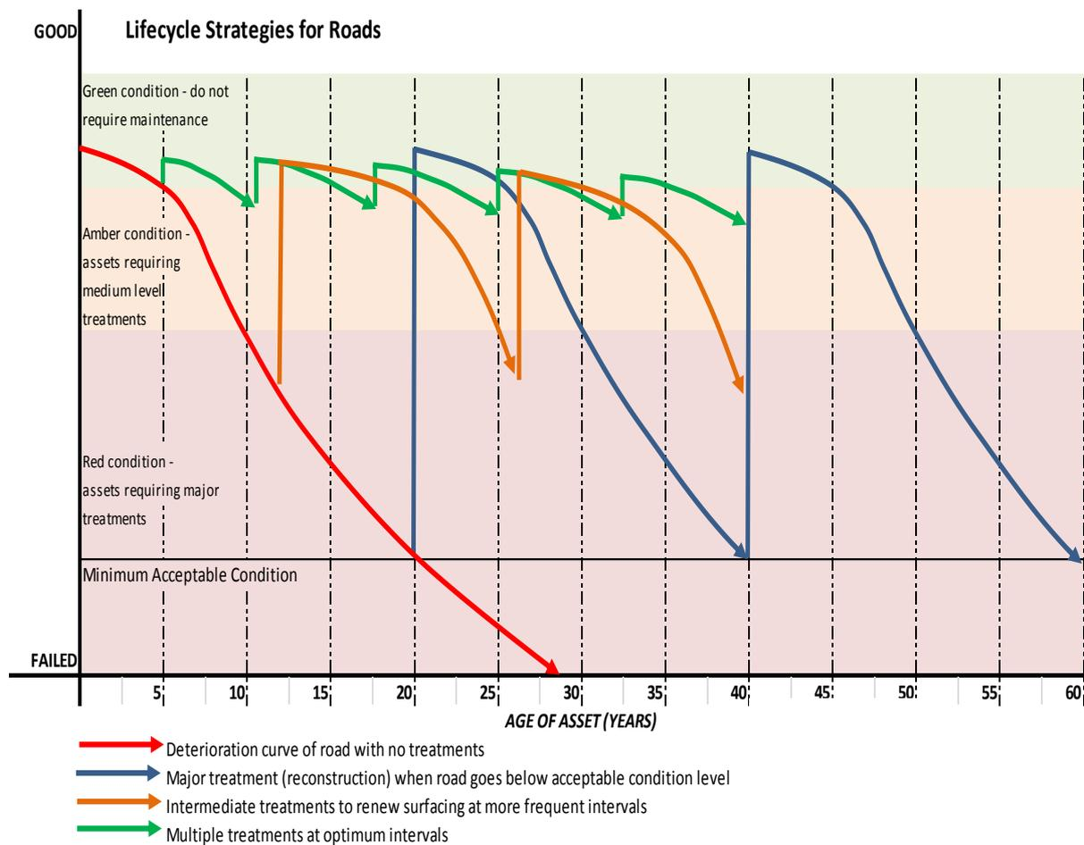
The red line shows how a road deteriorates from when it is constructed.
